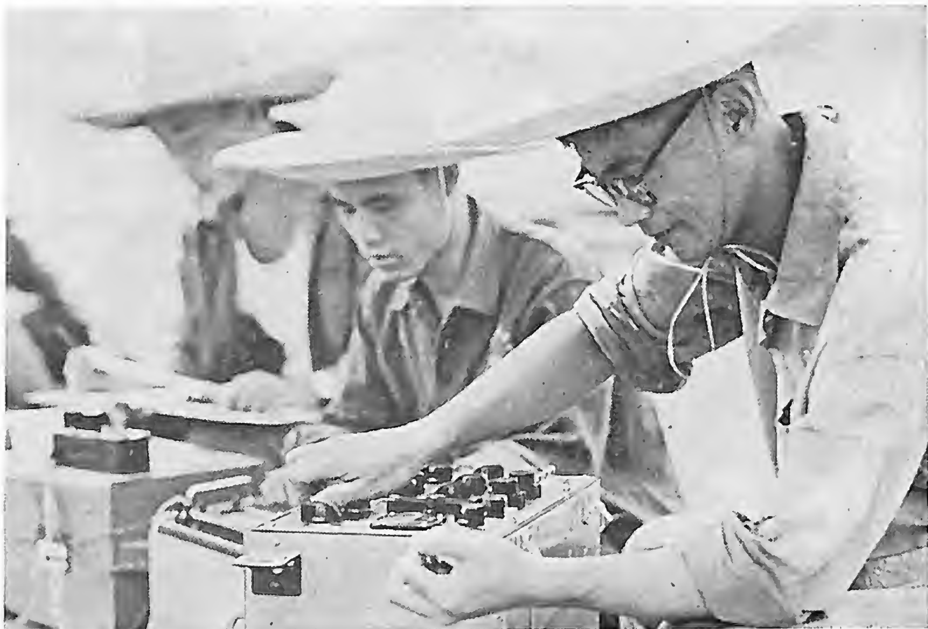
Surveying underground water by means of a potentiometer.
